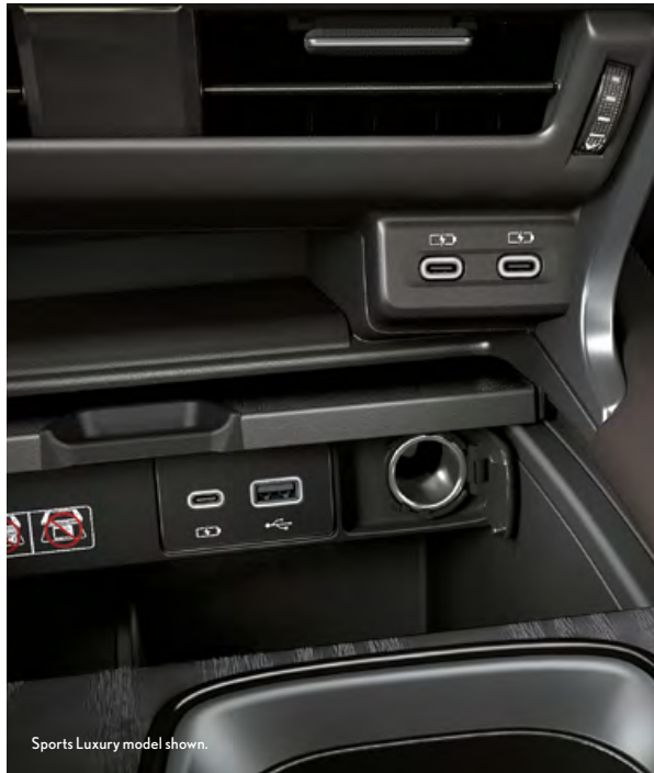
Centre Console: 3 USB Type C charging and USB Type A multimedia communication ports, DC12V
